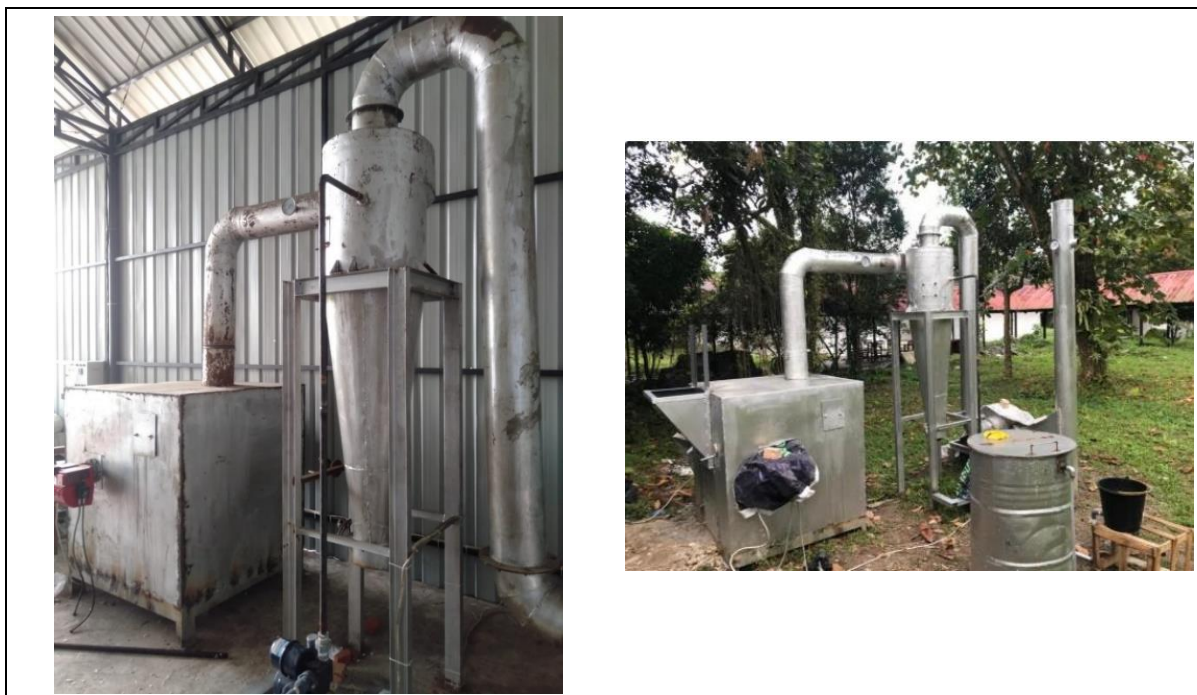
1a. The incinerator as a result of Dr. Eng Hafizhul Khair et al to process domestic waste
