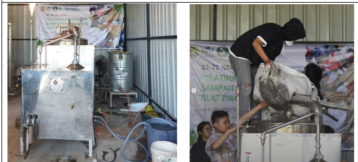
1b. Pyrolysis equipment which is a grant from Earthwise Consulting Japan to process plastic waste into fuel oil
