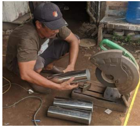
Gambar.4.2.b Pemotongan pipa Stainless Steel
