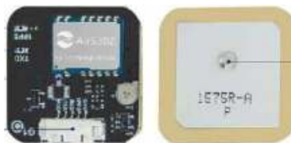
Gambar 8 Modul GPS Air530z
